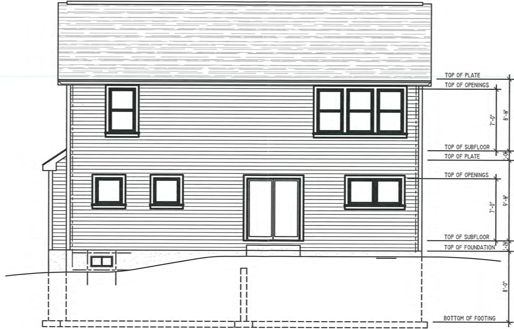
WEST ELEVATION SCALE: 1/4"=1'-0"
