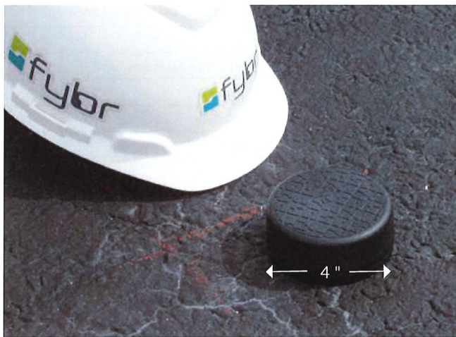
Fybr's parking sensor shown before it is core drilled into pavement.
