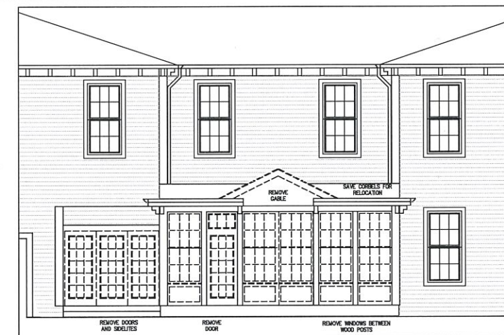
EXISTING/DEMO SOUTH SIDE ELEVATION Scale: 3/16" = 1'-0"
