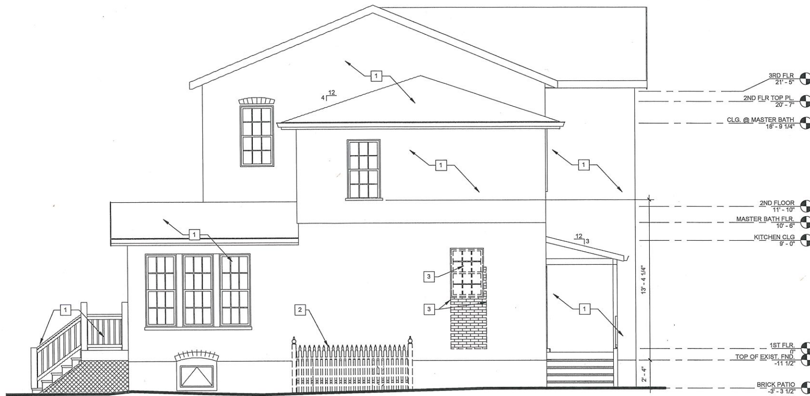
1 EXISTING / DEMO WEST ELEVATION AB 1/4" = 1'-0"
