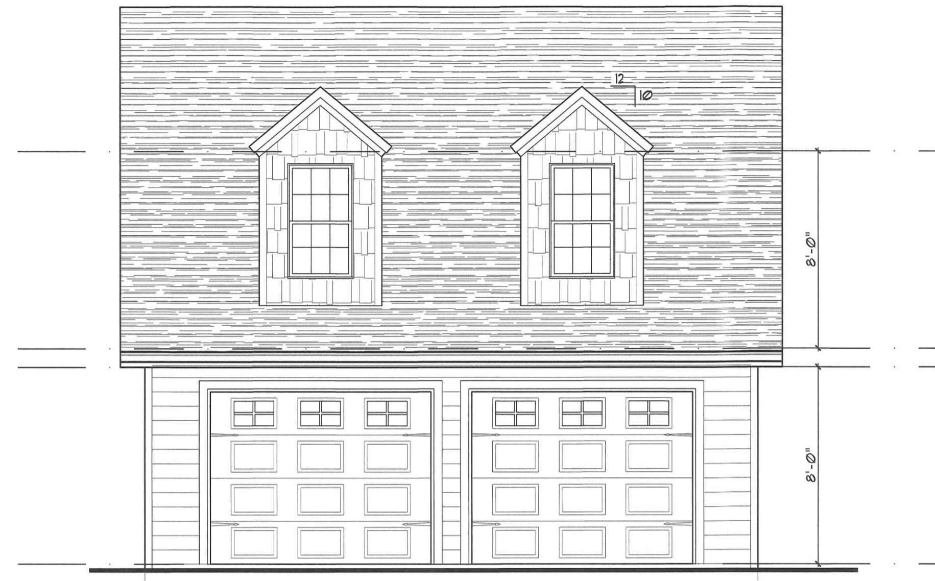
C FRONT ELEVATION 1/4" = 1'-0"
