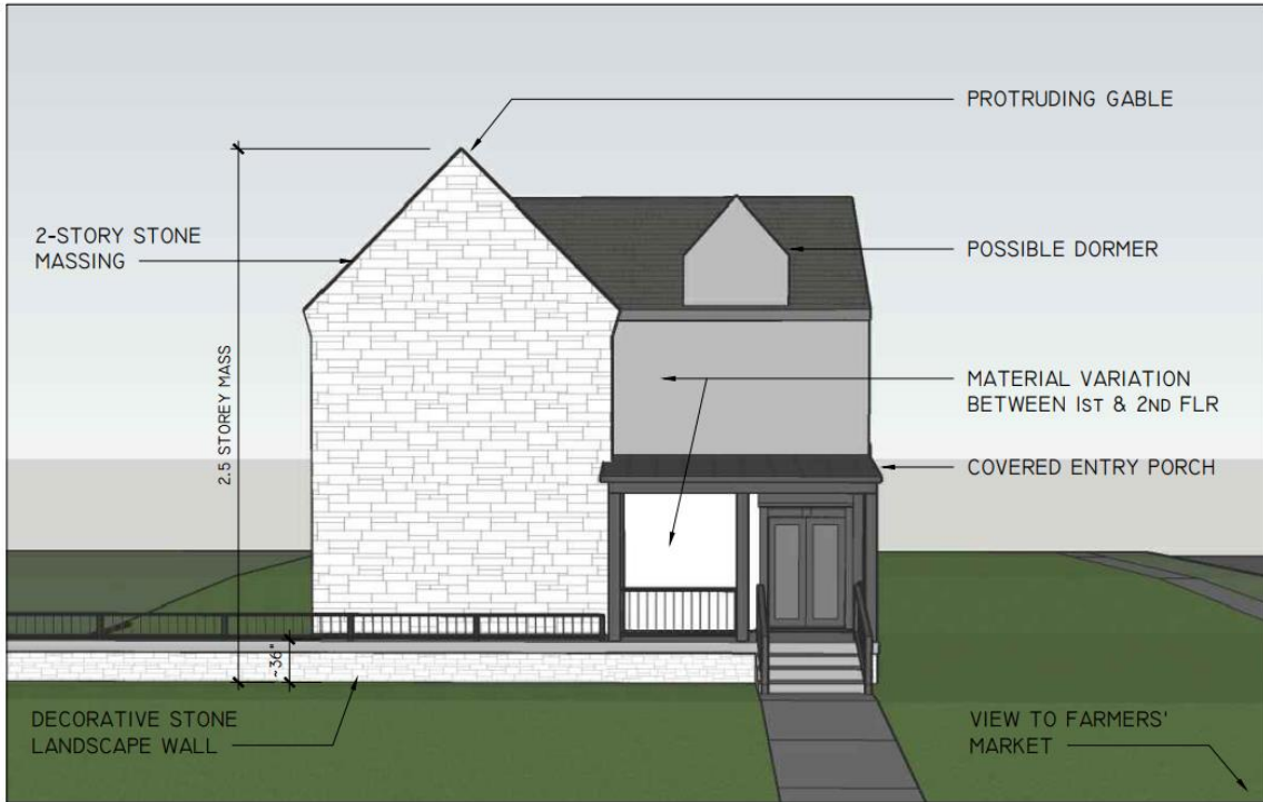
1 DIAGRAMMATIC MODEL OF PROPOSED HOUSE AS SEEN FROM WEST (TAYLOR) - SECOND ITERATION A.X SCALE: NTS
